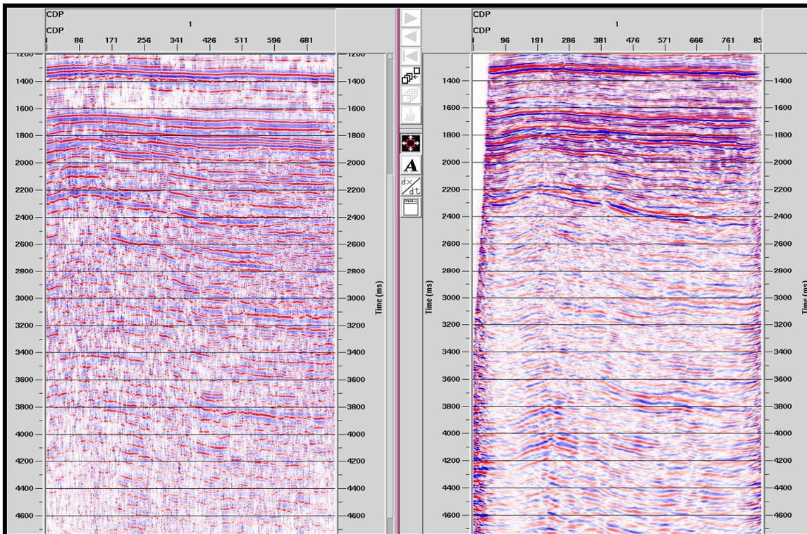
Figure-5: Comparison of earlier processed section and reprocessed PSTM Image
