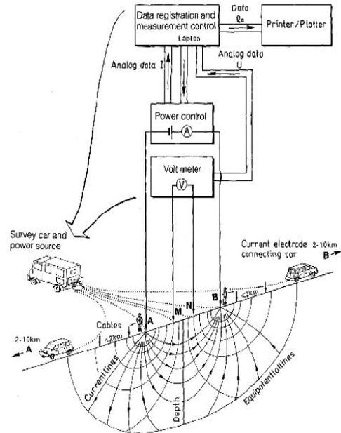
Figure 2: Schematic Field layout of Schlumberger Sounding method.
