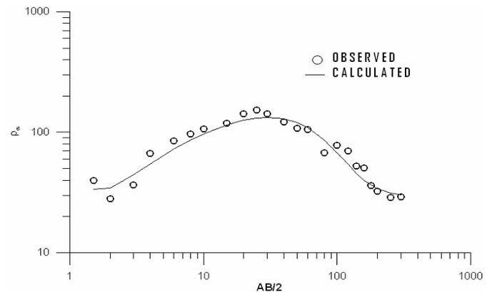
Figure 4: Sounding Curve representing observed and calculated data
