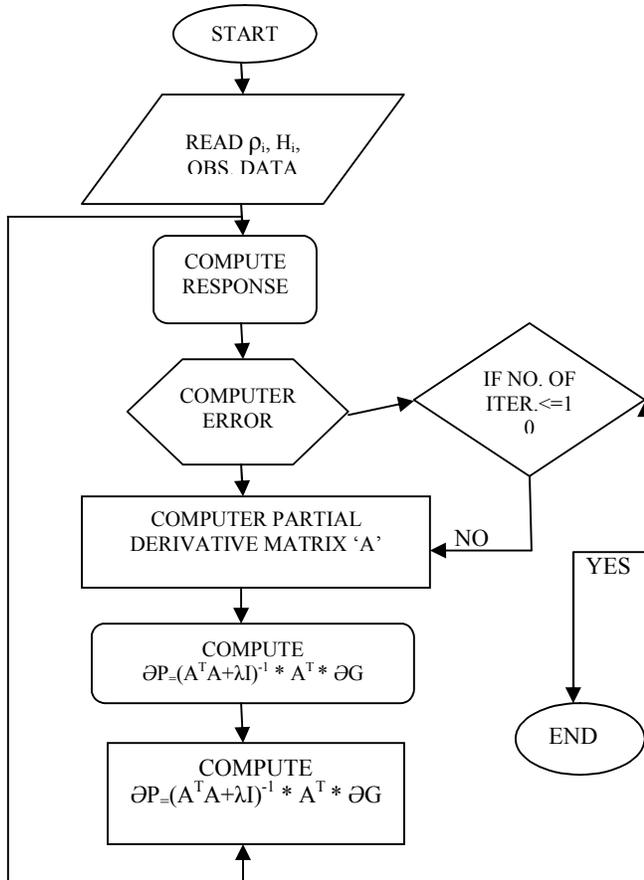
Figure 3: Flow chart of forward modeling algorithm
