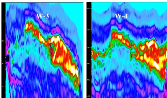
Figure-7: Lithology predicted for Well-3 & 4 agrees with drilled data
