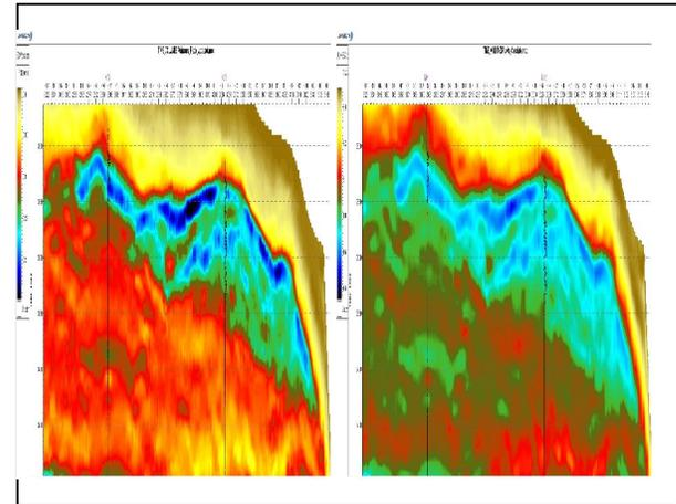
Figure-4 (a) Poisson's Ratio (b) Vp/Vs clearly outline the reservoir geometry.
