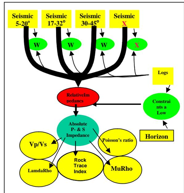
Figure-2: Generalized Work Flow for Simultaneous Angle Dependent Inversion (SADI). The inputs are angle stacks, derived wavelet corresponding to each angle stacks, Constrained log derived low frequency model. The output attributes : P-Impedance, S-Impedance, Vp/Vs, Poisson's ratio, Lambda-Rho & MuRho.
