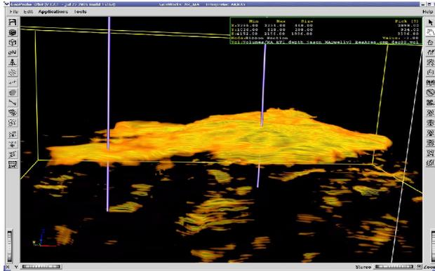
Figure-6 Geobody Captured using RTI cutoff delineates the reservoir extent
