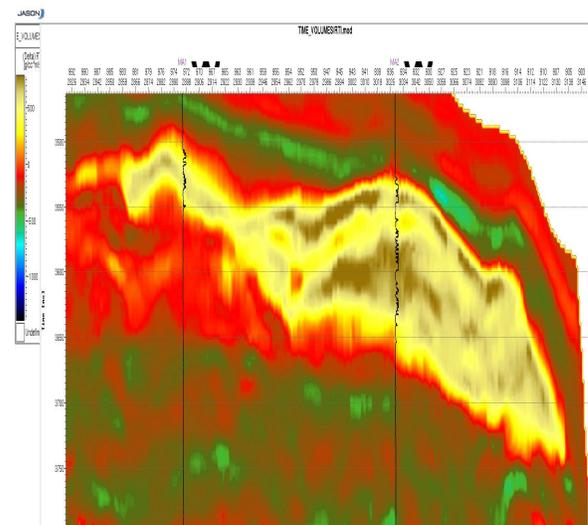
Figure-5 Rock Trace Index(RTI) identifying fluids and lithology
