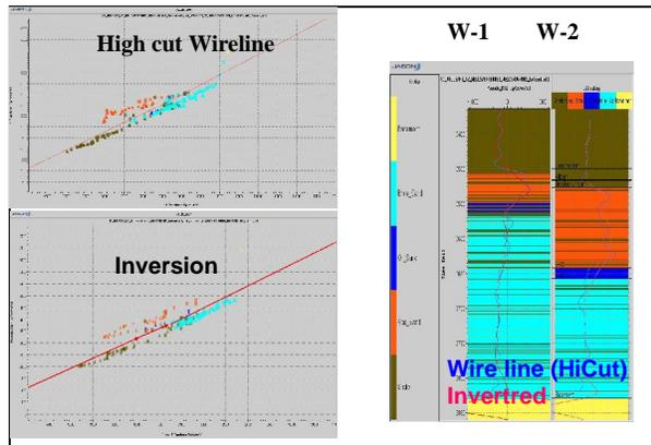
Figure 3a: Cross plot PI & SI using high cut wire line log data and Inversion data .
