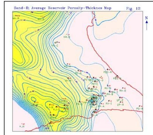
Figure 12: Porosity- Thickness Map of Sand-B
