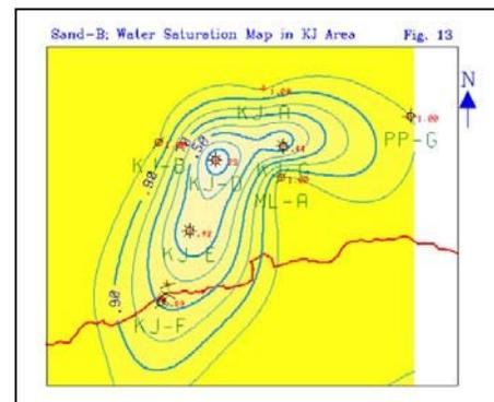
Figure 13: Water saturation Map of Sand-B in KJ area. Yellow colour represents high water saturation.
