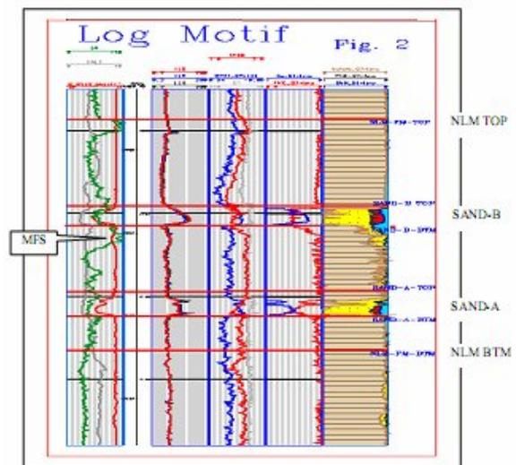
Figure 2: Log motif showing different sand units. Green & red traces in 1st track are GR & SP log; 2nd & 3<sup>rd</sup> track shows resistivity & porosity logs; 4<sup>th</sup> & 5<sup>th</sup> track displays computed porosity,  $S_w$  logs & lithology with fluids respectively
