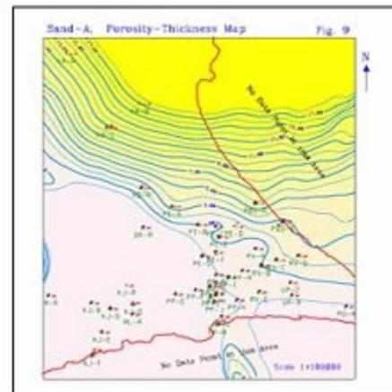
Figure 9: Porosity-Thickness Map of Sand-A
