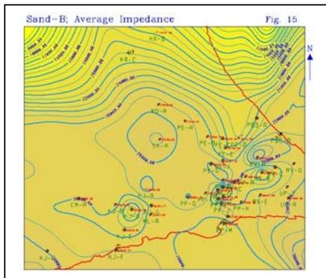
Figure 15: Average Impedance Map of Sand-B. Darker shades indicate higher values. Low values towards NW is due to shallow depth of burial
