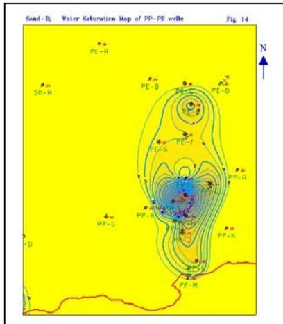
Figure 14: Water Saturation Map of Sand-B in PP-PE Area.
