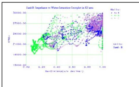
Figure 16: Crossplot showing variation of impedance with water saturation of Sand-B. Gas section shows lower impedance.
