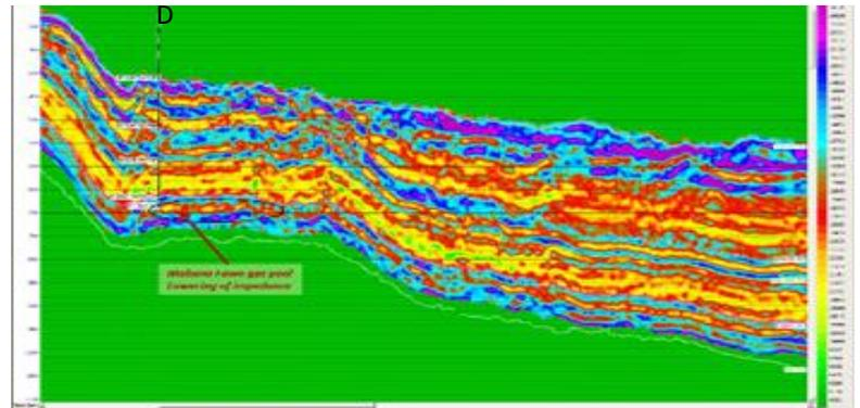
Fig.10 Impedance section along a 2D seismic line showing low impedance against gas bearing MF Limestone in well D
