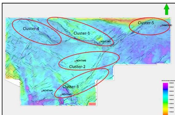
Fig. 11. Impedance map a window 20-60 m below the top of Mohana Fawn Limestone corresponding to gas bearing zone superimposed on the ant track derived fracture trend showing the prospective clusters
