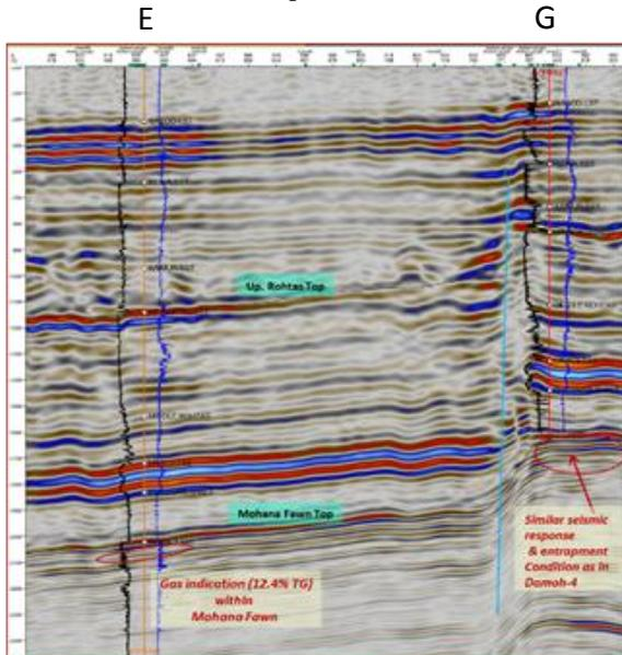
Fig.9. Arbitrary depth section (3D) showing zone with gas indication in well E (not tested) and G (MF Limestone not drilled).
