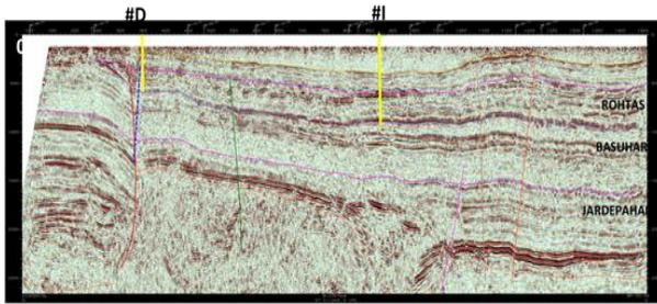
Fig 3. 2D Seismic section showing location of well D.
