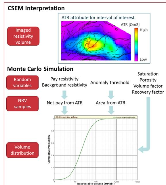
Figure 2: Illustration of the method for “Constrained EM positive” volumetric calculation.
