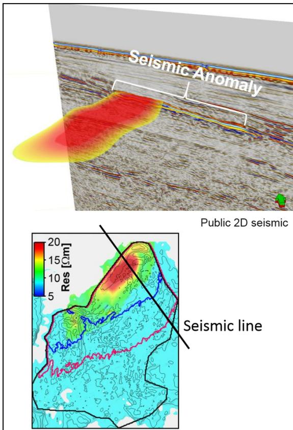
Figure 6: 3D CSEM inversion result of the Pingvin prospect co-visualized with the seismic line (top) and average vertical resistivity map displayed with contoured reservoir thickness from
