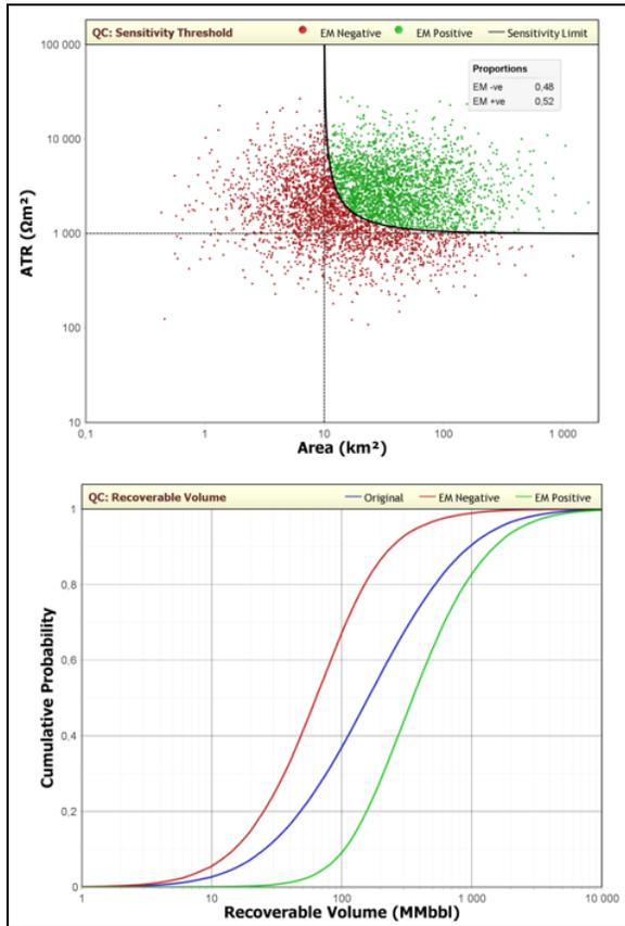
Figure 1: Sensitivity classification of reservoir realizations into “EM positive” and “EM negative” cases (top) and resulting update to the original/prior volume distribution (bottom). ATR describes the Anomalous Transverse Resistivity of the prospect defined as the product of *pay resistivity contrast* x *net pay*.
