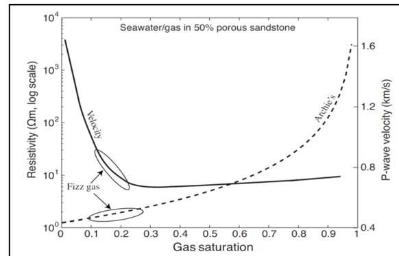
Figure 4: Resistivity (dashed) has good sensitivity to hydrocarbon saturation, while seismic velocity (solid) can typically only distinguish between presence and absence of hydrocarbons. From Constable (2010).
