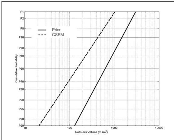
Figure 5: Prior and post-CSEM Net Rock Volume (NRV) distribution for the Pingvin prospect.
