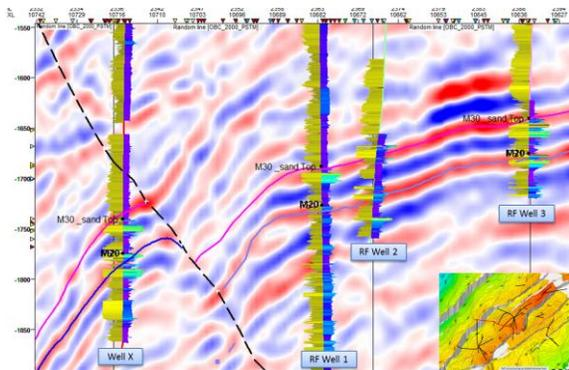
Fig.9: Seismic section along Well X and main field RF area wells.
