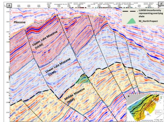
Fig.7: Seismic section in dip direction along RE-North prospect area showing stratigraphic setup.
