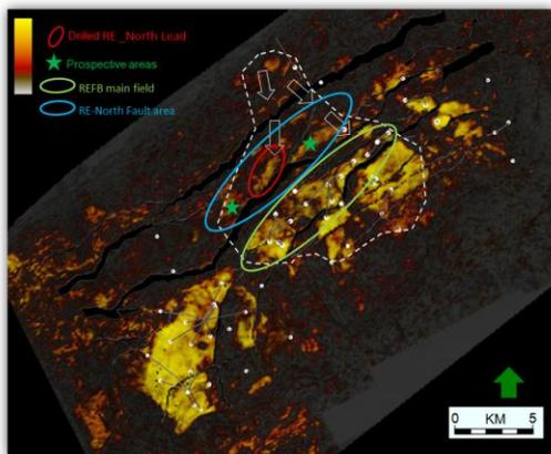
Fig.3: Geobody at Middle Miocene level showing depositional trend.
