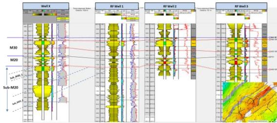
Fig.8: Well X log section showing various sands encountered and its correlation with main RF area wells.
