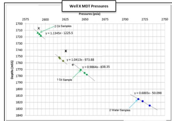
Fig.10: MDT pressures with sample points.
