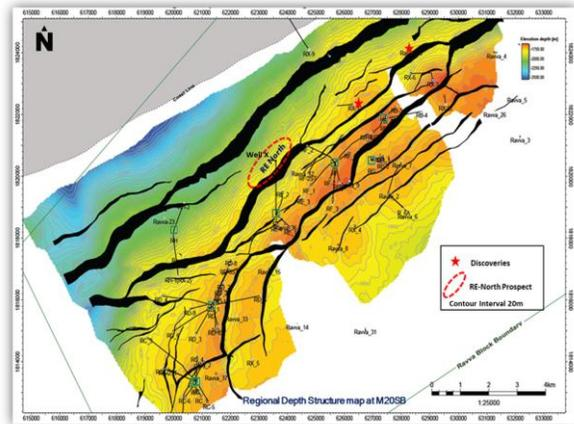
Fig.6: Depth Structure map at M20SB level showing structural setup of RE-North prospect.
