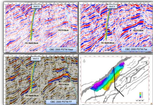
Fig.5: Section along RE-North Prospect and the main REFB Field showing AVO effects by comparing Near and Far seismic stacks. A Fluid Factor section is also shown along the same line showing brightening across hydrocarbon bearing areas.
