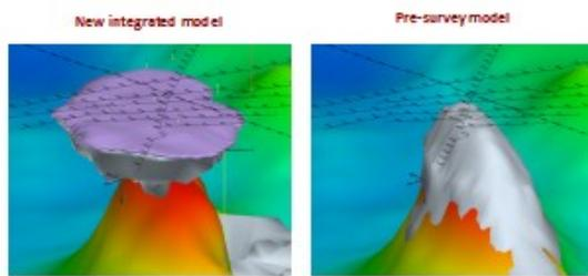
Figure 4: Example of a subsalt interpretation using magnetotellurics. On the right side is the interpretation without the magnetotellurics (MT) and on the left after the MT survey, interpretation and integration (After Buehnemann et al., 2002).
