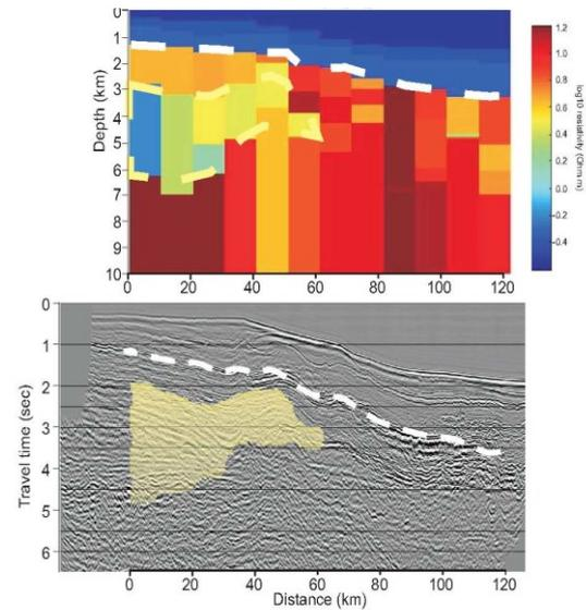
Figure 2: Example of joint inversion of magnetotelluric, gravity and seismic data (Jegen et al., 2009). The top diagram shows the joint inversion of gravity and magnetotelluric data and the bottom after seismic was used to constrain the inversion.
