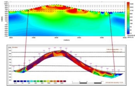
Figure 3: Examples section of magnetotellurics and DC resistivity data for complex terrain (Zerilli, 2002). The top shows the magnetotellurics section and the bottom the DC resistivity section.
