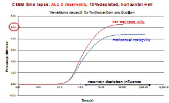
Figure 6: Percentage difference for vertical and horizontal resistivities for a horizontal well in the Bakken with 10% depletion. The anomalous response is still in the order of 5%.
