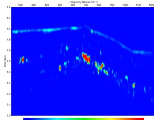
Figure 4: Teager-Kaiser energy section at 35 Hz frequency from TFCWT processing. Compare this section with 35 Hz frequency image in Figure 2.
