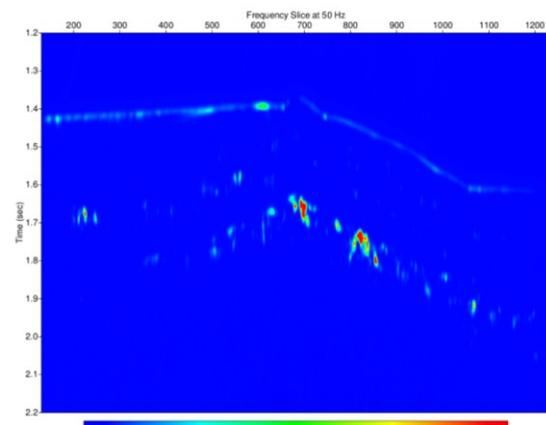
Figure 5: Teager-Kaiser energy section at 50 Hz frequency from TFCWT processing.
