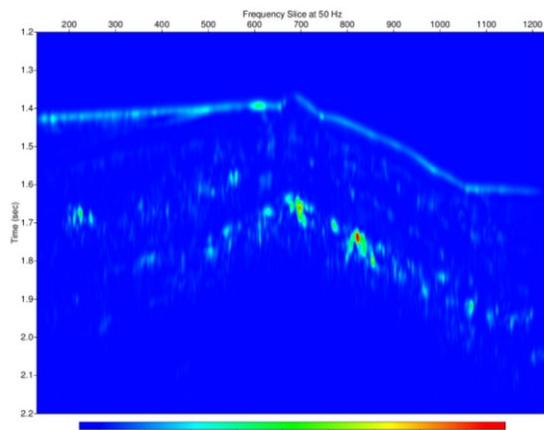
Figure 3: 50 Hz frequency image from TFCWT processing. Energy below BSR diminishes. Compare this section with 35 Hz section in Figure 2.
