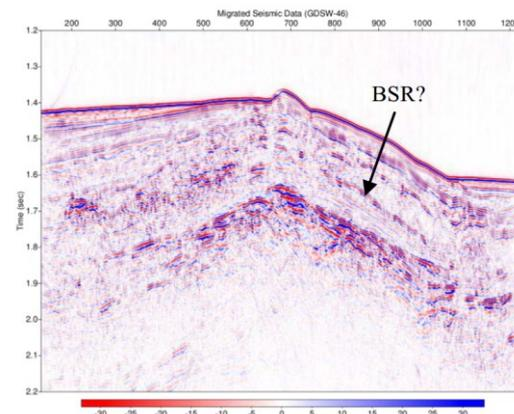
Figure 1: Migrated 2D seismic section in KG basin. Zones above the BSR have gas hydrate accumulations that has been confirmed by NGHP drilling.
