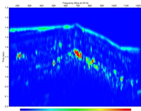
Figure 2: 35 Hz frequency image from TFCWT processing. Illuminated zones below BSR are likely to have free gas accumulations.
