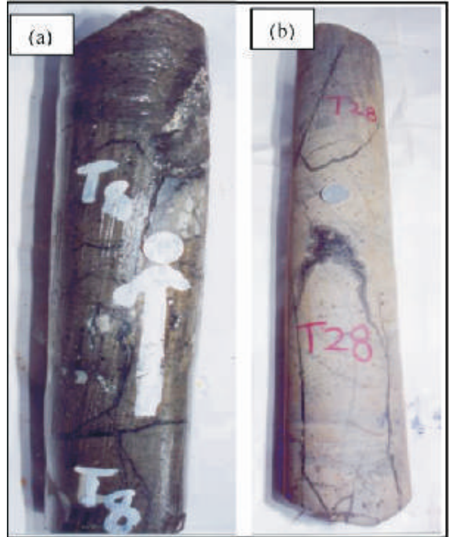
Fig.8: Core photograph of Deccan basalt. Core from depth 700.5 - 708m, recovery 81.7%, hard dense basalt with sub horizontal and sub vertical fractures filled with secondary minerals and dead oil (a). Core from depth 714.5-722, recovery 100% altered basalt showing numerous fractures filled with dead oil and Bitumen (b).
