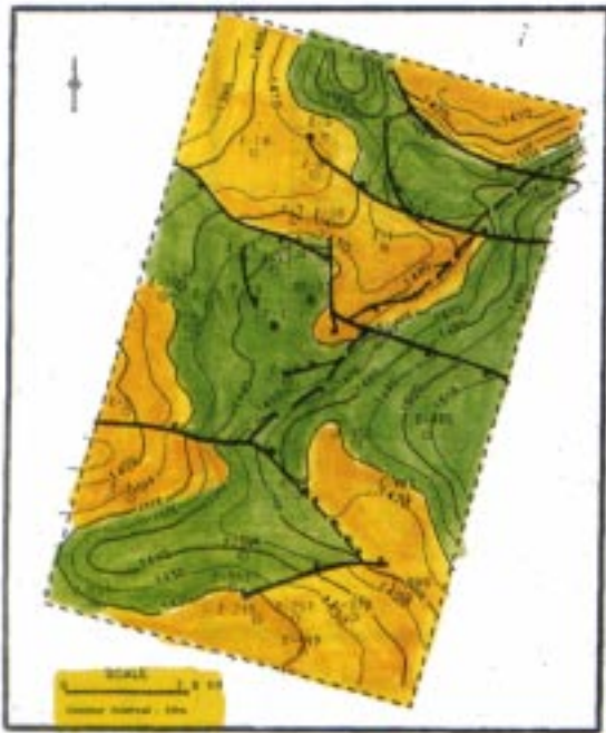
Fig 5. Depth structure map at K-IX horizon (yellow color indicates high and green color indicated lows and terrace feature).
