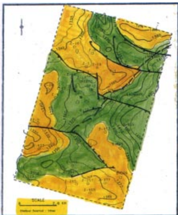
Fig 4. Time structure map at K-IX horizon(yellow color indicates a high and green color indicates lows and terrace feature).
