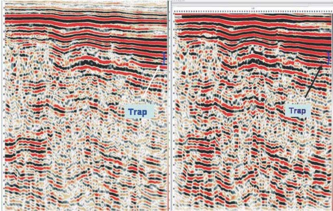
Fig.3 Comparison of Kirchhoff PSDM, on left (17 Hz) v/s RTM PSDM (17 Hz)
