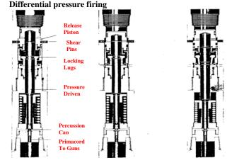
Before firing after shearing pins after firing
